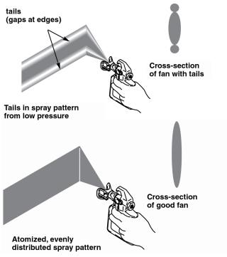
Spray tip wear is common with airless spray applications and any wear should be monitored and spray tips should be replaced when necessary. Using worn spray tips will increase pressure losses in spray hoses as well as applying heavier than recommended film thicknesses.
